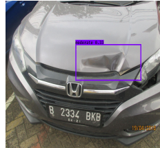
Dent and intensity of impact detection for repair cost evaluation
